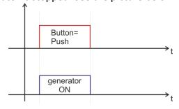
**LATCH-** pushing the button once the generator starts, pushing the button again the generator stops.
