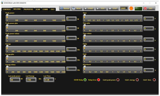
Before setting the welding regime you need to Select TRIGGER Mode for the button – you can do it in PROPERTIES Tab or from the Display.
